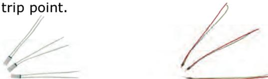
Thermal protection cut outs can also be built into the windings, bearing housings of motors and fitted to compressors as over or under temperature as part of the shut down circuitry.
