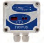
Other parameters such as signal input type, logging interval, etc, are easily selected through the LogChart-II software. Inputs RTD, Thermocouple Types K,J,T,N,R,S,B 4- 20 mA , 0-20 mA & 0 -10 V
