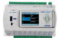
**FieldLogger** has one USB interface to be connected to a computer (for configuration, monitoring and data download) and another USB port for plugging a flash driver for data retrieval. The 512k logging basic memory is used to store data and it can be greatly expanded with an SD card
